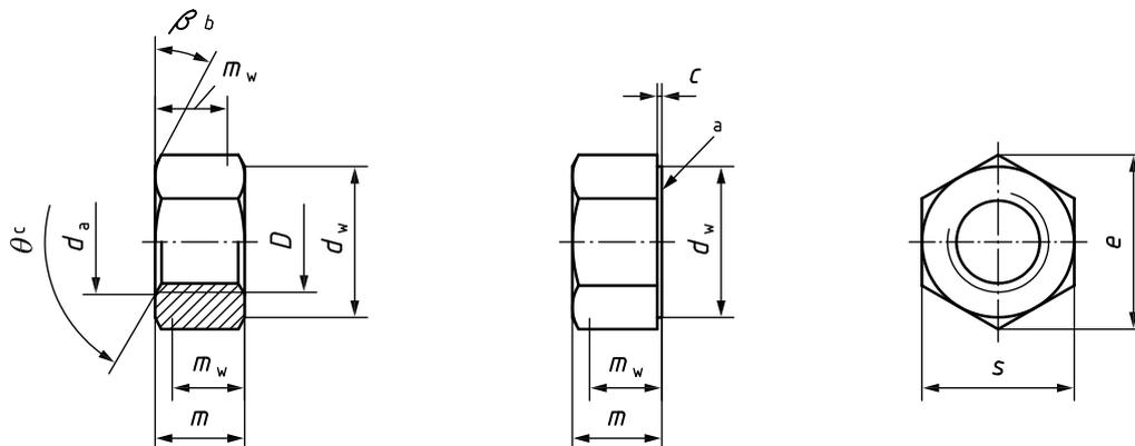
a Unless otherwise specified at the time of order, the nuts are delivered without washer-face.
